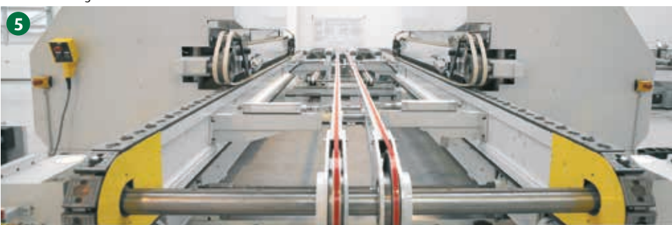
5 Definition of profile length in the double-end profiling machine
