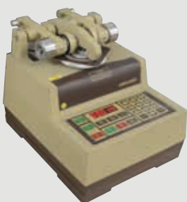
Test of abrasion resistance using the Taber Abraser
