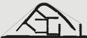
Combi-Pack FN lock-on aluminium stair profiles (flooring profile, installation system, screws and dowels, Adapter profile)
