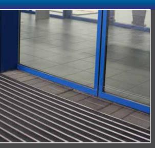
L45 is our low profile system, with body height of 8 mm and total height 12-14 mm. It comes with a ramp profile for "on top" installation. The width of the profiles is 45mm, while the inserts are 22mm. The closed construction does not allow dirt to fall under the mat, hence no need to lift the mat for cleaning.
